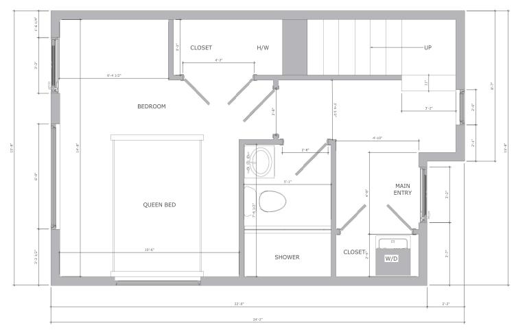
NOTE: EXTERIOR DIMENSIONS INCLUDE 1/2" SHEATHING, INTERIOR DIMENSIONS TO FRAMING
