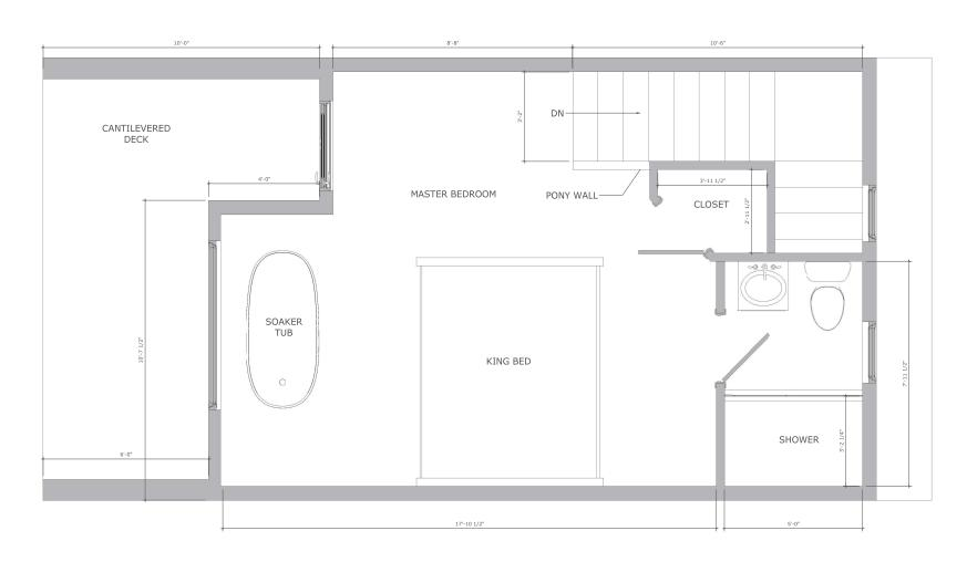
NOTE: EXTERIOR DIMENSIONS INCLUDE  $1/2^{\prime\prime}$  SHEATHING, INTERIOR DIMENSIONS TO FRAMING
